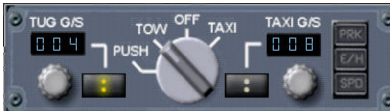
Tow mode engaged at with desired tug speed set at 4 kts.
